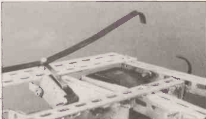
Picture 2: One of eight microswitches used to provide all-round touch sensing on a small robot
